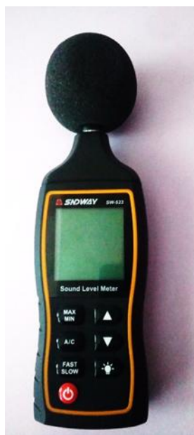
Figure 1. Class 2 Sonometer used in the study
